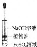
A 观察  $\text{Fe}(\text{OH})_2$  的生成
